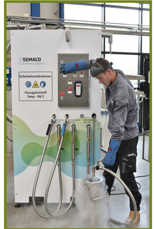
Filling an open dewar manually
