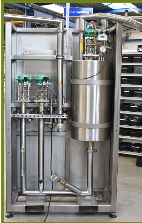
Back view filling station Type 4.
