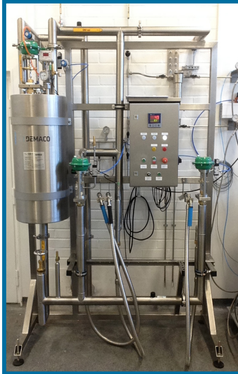
Filling station with vacuum insulated valves
