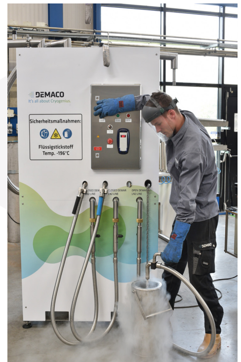
Filling an open dewar manually
