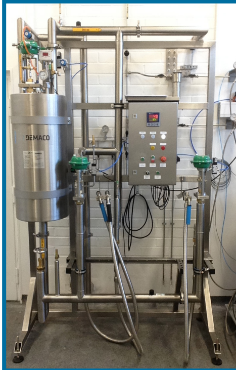
Filling station with vacuum insulated valves
