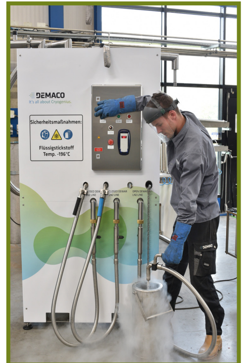
Filling an open dewar manually
